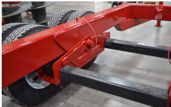
Tandem Axle Walking Beam Supreme's walking beam is designed to distribute and carry the weight of the mixer through the tandem axle easily and effectively. Available on 900T-1900TR.
