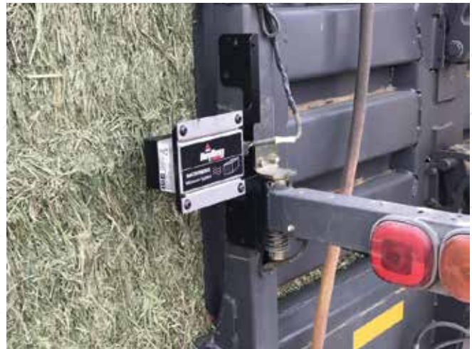
Microwave sensors mounted on the rear of the bale chamber.
