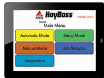
The HayBoss 600 Series Automatic Applicator can be controlled with an iPad or iPad mini, or can be displayed through the tractor ISOBUS display.
