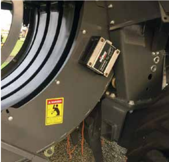
Microwave sensors mounted on the baler pre-compression chamber.
