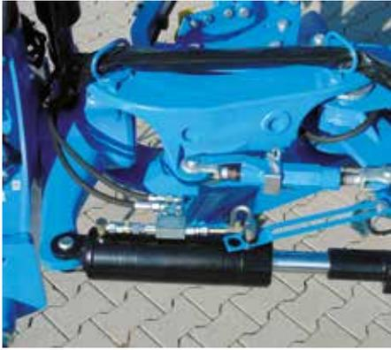
The new TurnControl significantly improves the turning process of the plough.
