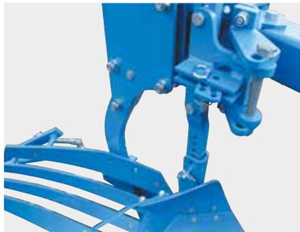
mers on the plough are set uniformly without the need for further alignments or measurements. The angle is unchanged as depth is amended.
